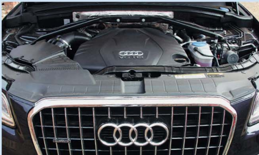
▲ Cutting-edge common-rail TDI diesel V6 puts out 580 Nm of torque
