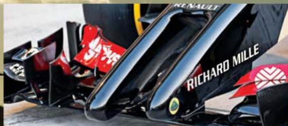
▲ Unique nose design on the Lotus-Renault E22 race car
