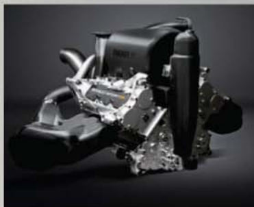
▲ Manufacturers go full-blown this year with turbocharged V6 engines
